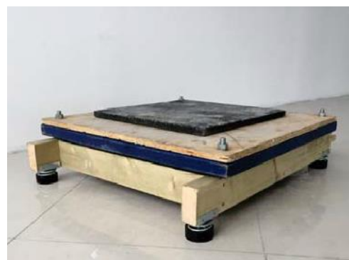
Figure G5: Floor 3 - 4Hz sprung floor system + 50mm rubber mat rubber. Floor 4 - 6Hz formwork sprung floor system + 27mm rubber
